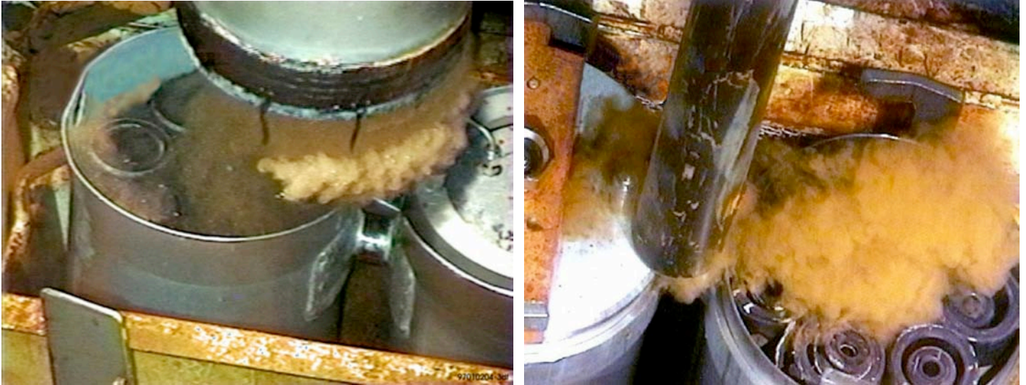
Residual Sludge from Corrosion of Spent Fuel is Stirred up During Fuel Retrieval in K Basins
