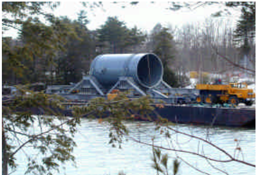
Shipping Container for Maine Yankee Reactor Pressure Vessel
