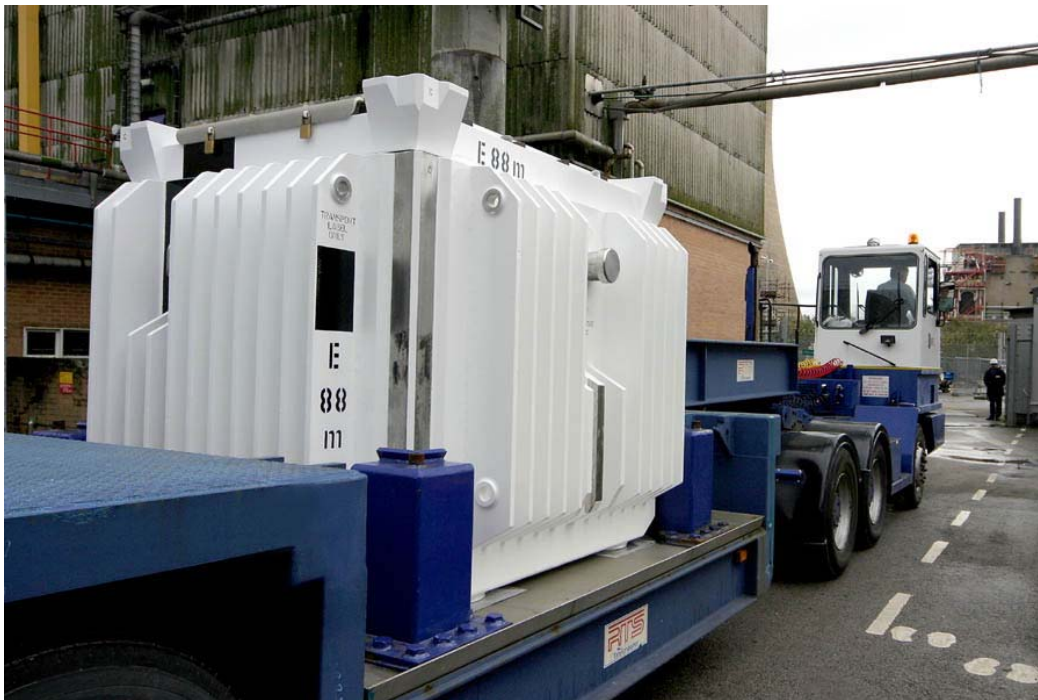
The retrieved Magnox fuel skip within a 50-ton transit flask leaves the legacy pond
