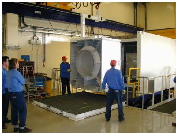
The Gemini container used for moving PCM items from the low level waste repository to Sellafield
