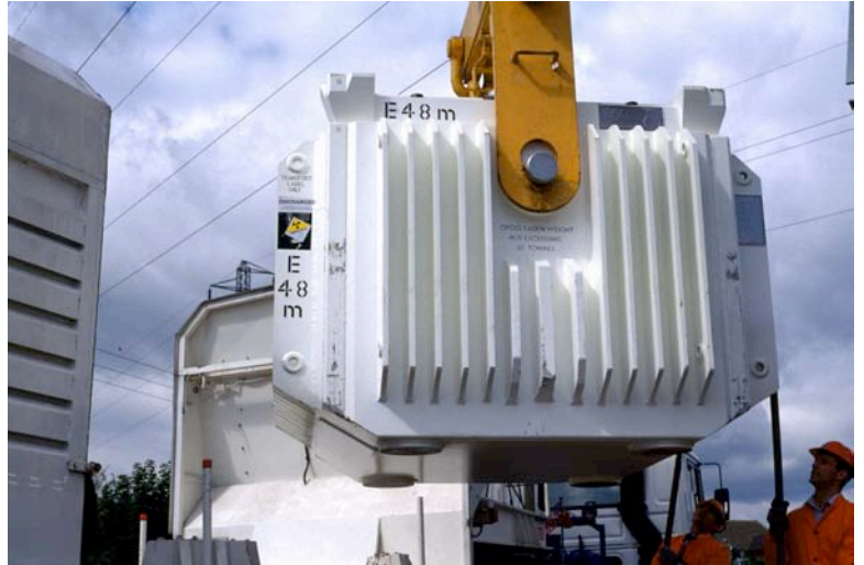
Transferring the 50 ton flask containing around 200 fuel elements to a railway flatrol
