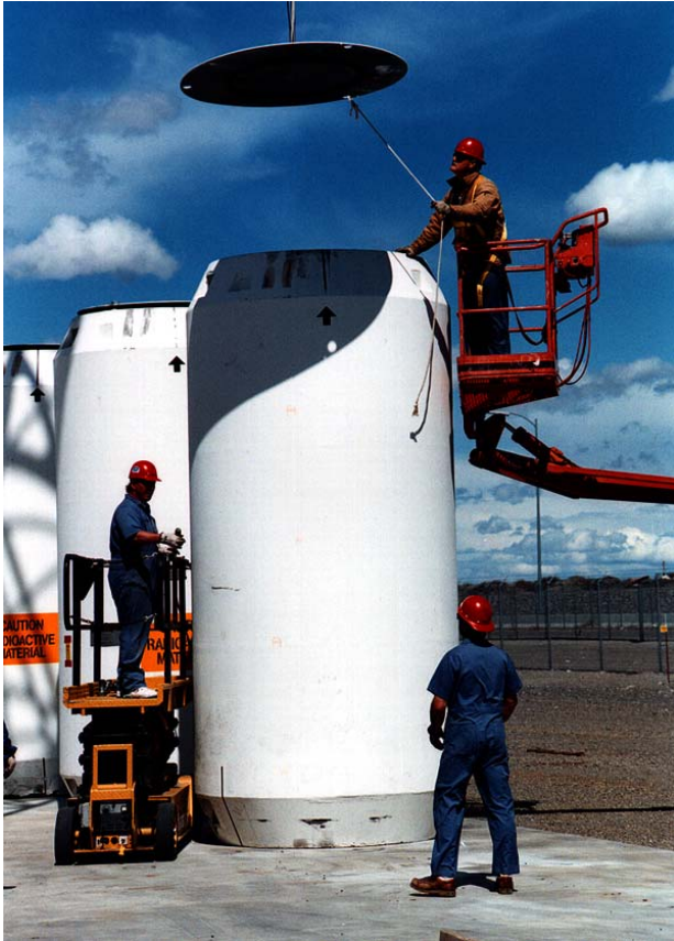
Interim Storage Cask (ISC) for Spent Fuel Assemblies
