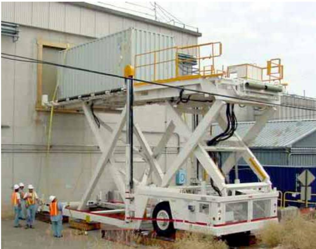
**The modified MDL-40 allows crews to load waste directly into a cargo container from the 2<sup>nd</sup> floor**
