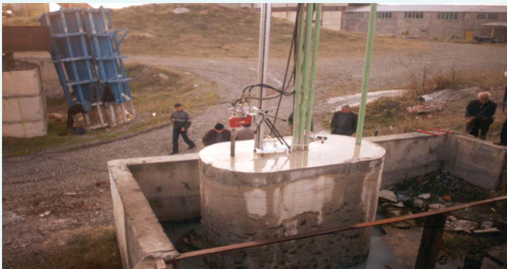
Fig 3 Mock-up of Georgia's reactor to simulate entombment
