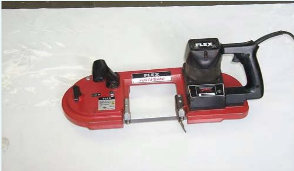
Fig 2 Handheld mechanical cutting equipment for small contaminated pipes, BR-3 decommissioning project, Mol, Belgium
